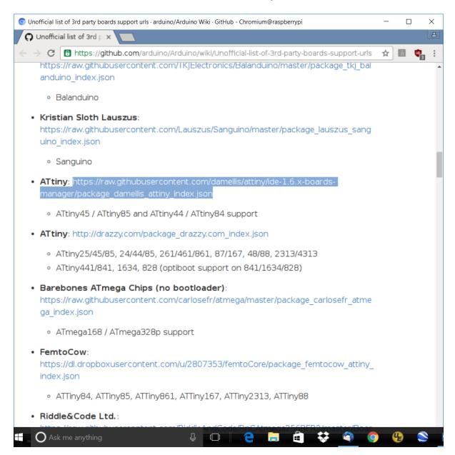
2.13 Copy the url (<a href="https://raw.githubusercontent.com/damellis/attiny/ide-1.6.x-boards-manager/package\_damellis\_attiny\_index.json">https://raw.githubusercontent.com/damellis/attiny/ide-1.6.x-boards-manager/package\_damellis\_attiny\_index.json</a>) and paste it into the dialogue at step 2.10 above. OK that dialogue. The Preference dialogue should now look like this:
