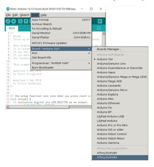
2.18 Return to the Board menu again and select the ATtiny84 processor (the clock should be Internal 1 MHz).
