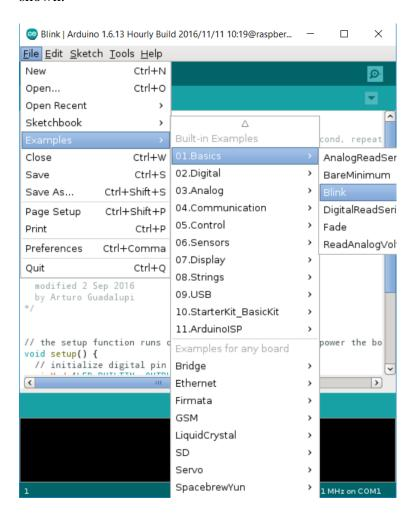
2.20 Edit the sketch so that it uses output pin 7 like this: (LED\_BUILTIN changes to 7 everywhere)
