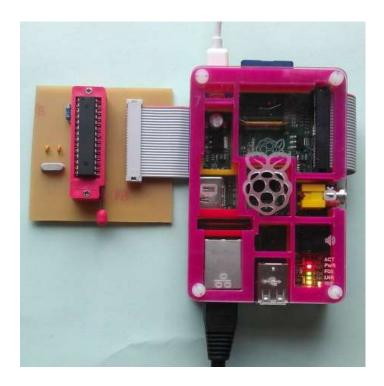
The scheme can also be implemented using a breadboard. This requires the chip to be plugged directly into the breadboard rather than by using a ZIF socket.
