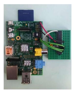
The final picture gives a close-up of how the jumpers are interconnected.
