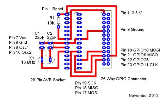
The above scheme has been implemented as a custom printed circuit board (shown below) using a ZIF (Zero Insertion Force) socket for the ATmega.
